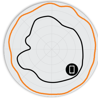
Figure 3. R650 5GHz Azimuth Antenna Patterns
