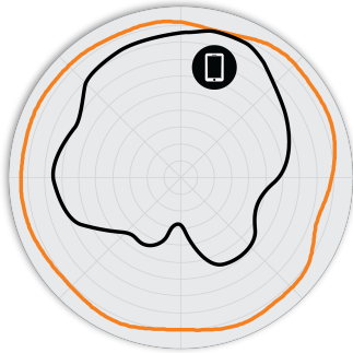
Figure 2. R650 2.4GHz Azimuth Antenna Patterns
